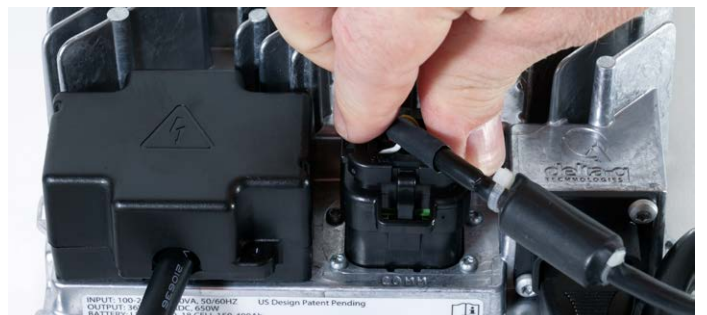
Figure 21. Apply pressure until you hear an audible “click” as the plug locks into position.
