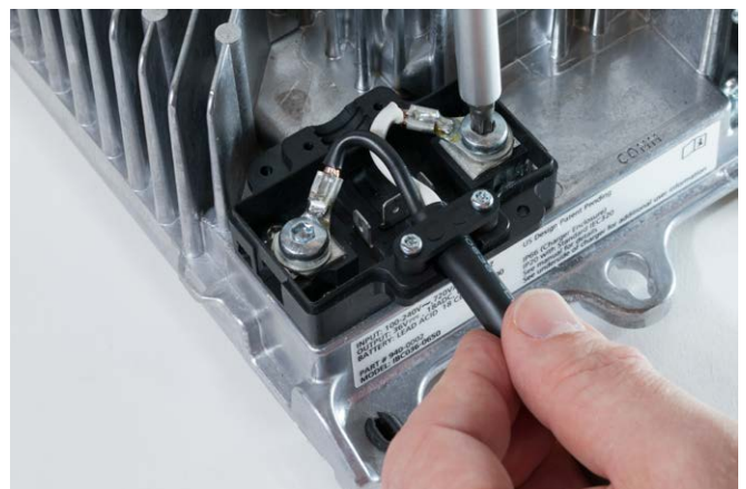
Figure 17. Fix the DC cable in place using the Delta-Q cable clamp, fastened with Torx T10 screws to a recommended torque of 0.6Nm +/-6%. Proceed by attaching the positive and negative leads to the positive and negative terminals, respectively, using the Torx T30 screwdriver and Torx T30 / M6 screws, with a recommended torque of 4.5Nm +/-5%.
